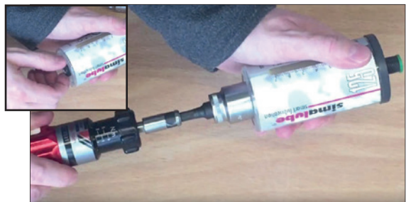
Screw in gas generator and tighten to 1.5-2.0 Nm
