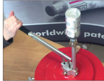
Fit the simalube onto the supply fitting and pump grease until it reaches the upper mark. ⚠ Do NOT overfill!
